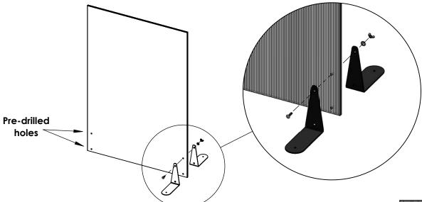
Insert bolt through top square hole in Metal Bracket and align with corresponding top hole in base of Divider Panel.
